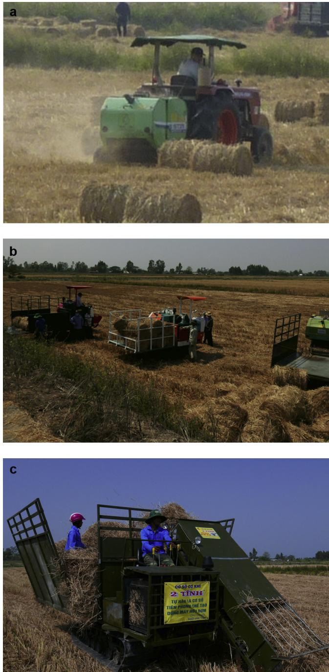
**Fig. 2.** (a) Roller baler pulled by a tractor. (b) Self-propelled balers. (c) Gathering machine (loose rice straw).
