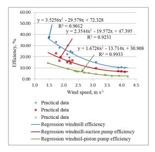
Figure 4 Efficiency of the system with different pumps
