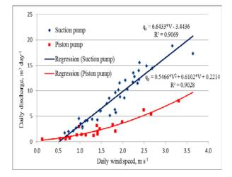
Figure 3 Discharge of the suction and piston pumps
