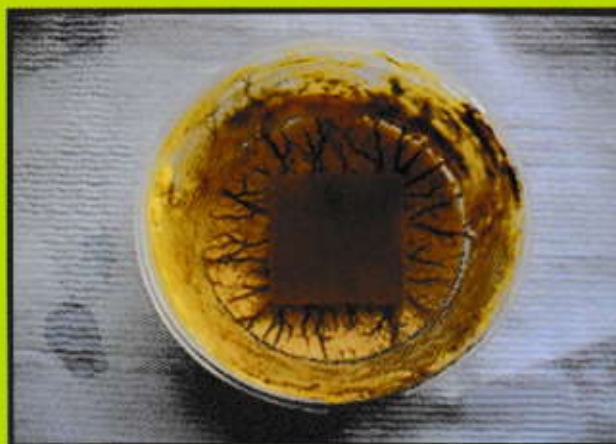
Plywood specimens after 16 weeks of incubation with C. puteana
