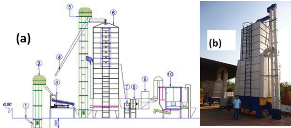
Figure 3. Recirculating columnar dryer (RCD), (a) schematic diagram and (b) photograph of the system in operation. 1 = Feeding, 2 = Bucket elevator, 3 = Pre-cleaner, 4 = Unloading pipe, 5 = Bucket elevator, 6 = Drying tower, 7 = Controlling component, 8 = Blower, 9 = Baffle, 10 = Furnace.
