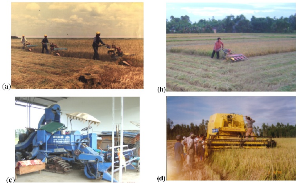
Figure 1: (a) Rice reaper, made by Long-An Mechanical Factory in 1985... (b) ... and one from 3 major reaper manufacturers remaining in 2004; (c) A combine made by a farmer-mechanics in Dong-Thap Province; (d) An imported combine under test in 1998.
