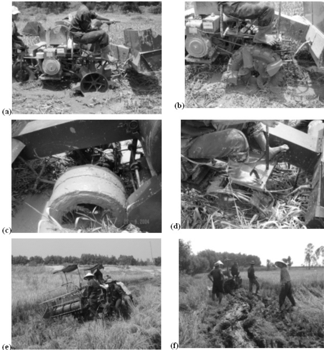
Figure 4: (a) The pyramid-shaped lug wheel; (b) Retractable lugs mounted adjacent to rubber tyre; (c) Dual tyre blocked with clay; (d) The cage wheel; (e) The combine is easily lifted for changing wheels; (f) Bogged-down combine on soft soil was simply pulled out by 7 people. (Tran V. Khanh et.al 2004).
