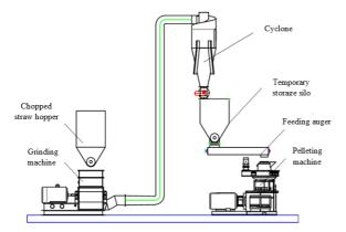
Figure 4. Schematic diagram of pelletizing system
