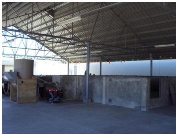
Figure 3. The SRA-8 dryer (8 tons/batch) used in the study
