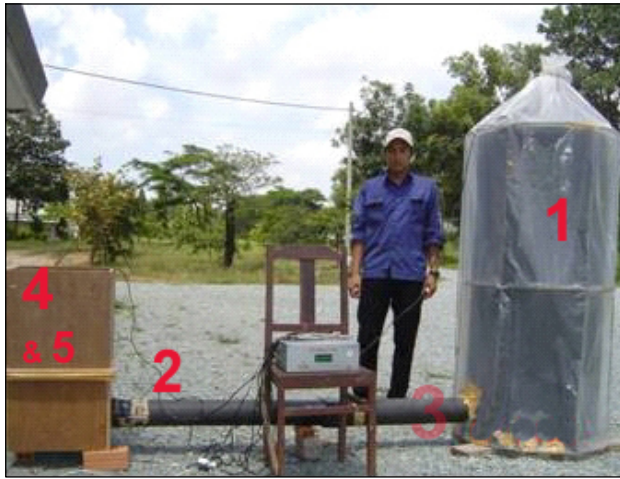
Figure 1. The laboratory dryer: (1) solar collector, (2) suction fan, (3) air duct, (4) drying chamber, and (5) trays.
